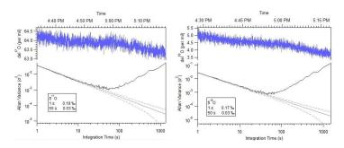
Instrument precision for a column density equivalent to 400ppm  ${\rm CO_2}$  mixing ratio and 36 meter optical path length.
