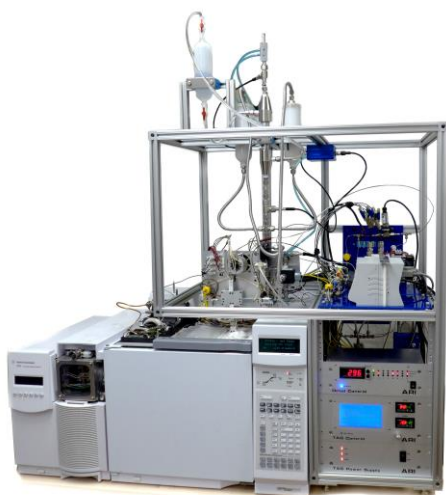
Stand-alone tag (with Agilent's 6890N/ 5975 MSD)
