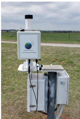
Cloud Properties Spectroradiometer deployed at Department of Energy’s Atmospheric Radiation Measurement user facility, Southern Great Plains site. The instrument is providing in-situ observational data to help better understand the role of clouds in controlling the Earth’s energy balance.
